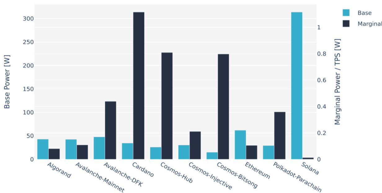
Figure 3: Base power demand and marginal power demand per TPS for a best guess single node of the respective network in watts.
